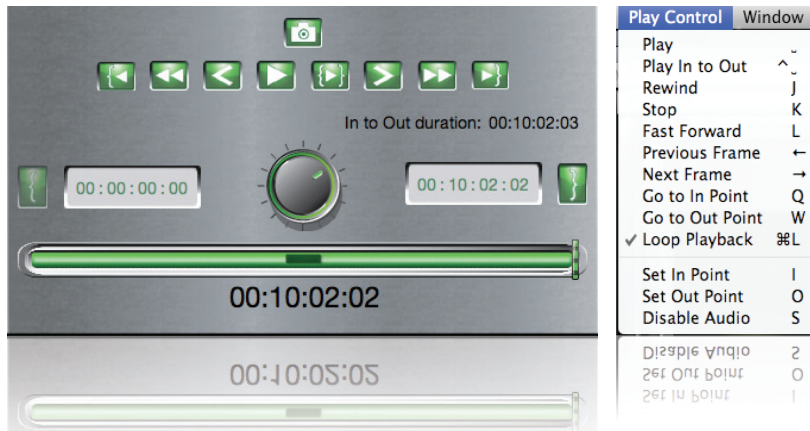
Matrox Vetura Playback controls – Play, Stop, Frame Forward (Step), Frame Rewind (Step) Fast Forward, Fast Rewind, Go to in-point, Go to out-point, Mark In, Mark Out, Scrub, Frame Grab, Loop, Mute, Audio Level Control with audio VU meters for up to 16 channels, Jog Control
